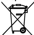
The actuator contains electrical and electronic components and must not be disposed of together with domestic waste.
